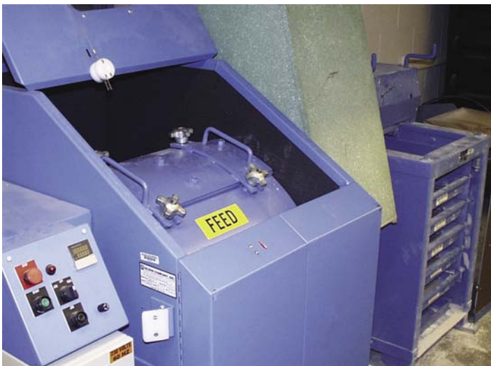
Figure 1. Hardness of aggregates for bases and pavements are often assessed using the Los Angeles Abrasion machine. Photo source: Southern Illinois University Edwardsville
