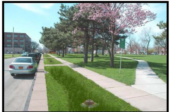
Urban Street After Rendering with Curb-side Bench, Grass Planting Bioretention, Underdrain with Overflow, Syracuse, NY
