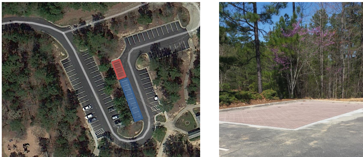
Figure 1. From left to right: (a) Aerial view of Piney Wood park: 540 ft 2 of PICP, 1635 ft 2 of contributing watershed area; (b) Piney Wood PICP retrofit.
