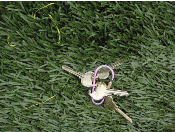
Figure PT-2.5: Permeable artificial turf (keys for scale). This material is typically laid over a base of washed open-graded aggregate.
